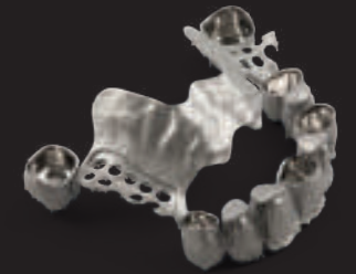
Milling results with high surface quality
